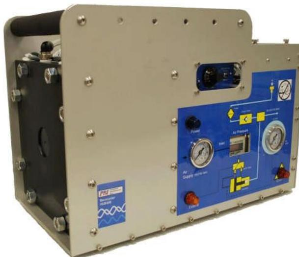
The Barocycler HUB440 is a compact, portable, bench-top, ultra-high pressure generator that uses compressed air-driven pressure intensifier to generate fluid pressure up to 58,000 psi (~4 kilobar) with an input compressed air pressure of just 130 psi. The HUB440 can be operated via a simple front panel, or controlled using the integrated Data Acquisition and Control Module for dynamic pressure control and connectivity to external devices.
