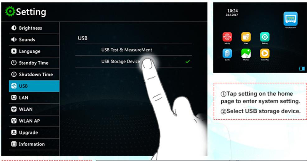
③Connect computer with USB cable to open Micsig file and can view saved waveform & screenshot.
