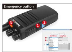
Configure your side keys 1, 2 and Emergency button using our simple CPS software to change functionality from changing zones to speaking power level, see documentation for more button features.
