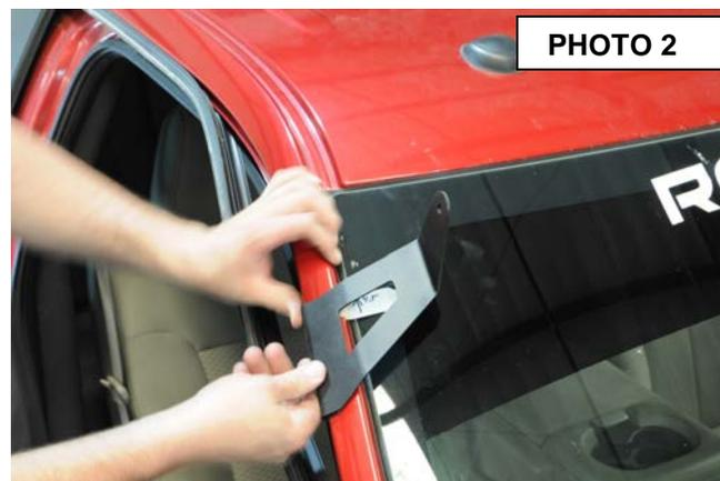
3. Use the supplied 3/16" rivets to secure the light brackets. **See Photo 3.** Repeat steps on the driver side.
