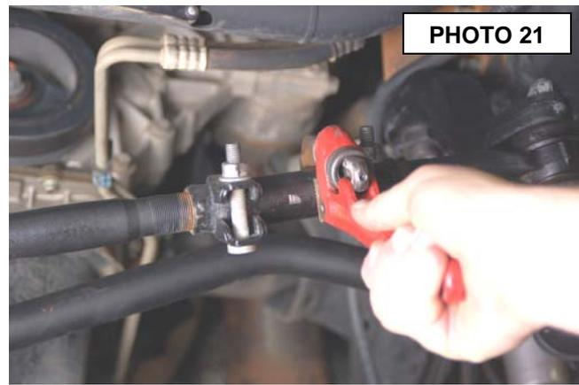
**IMPORTANT NOTE :** The draglink must be adjusted to the center steering wheel **BEFORE** the vehicle is driven. Failure to do so will cause a computer error, odd handling, and poor performance.
