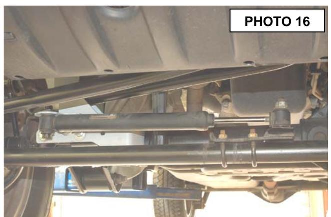
29. On the rear of the vehicle remove the factory sway bar link using a 18mm socket and wrench on the lower. Remove the upper hardware using a 18mm wrench and a 19mm wrench on the ball joint end.
