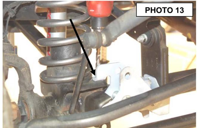
24. Tighten all 3/8" hardware using a 9/16" wrench.
