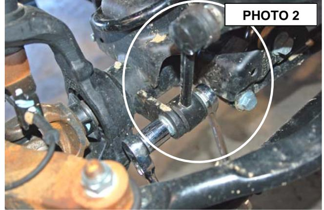
6. Remove the lower shock bolt using a 18mm socket and wrench. Using a 14mm wrench unbolt the top of the shock and remove. **See PHOTO 3.** Retain stock hardware.
