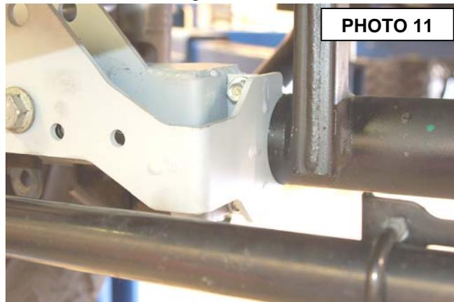
22. Install the two 3/8" x 1 1/4" bolts, washer and nuts in the new bracket and supplied stabilizer bracket if reusing the stock stabilizer in the far left holes as shown. If not installing the stock stabilizer, the two 3/8" x 1 1/4" bolts will be installed in the two far left holes in the bracket with out the supplied stabilizer bracket. **See Photo 12.**
