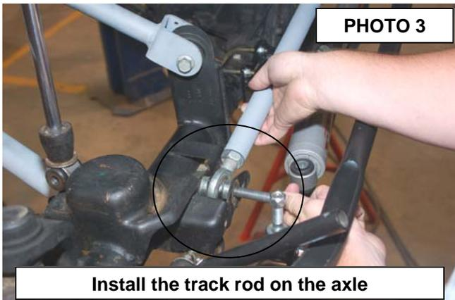
3. Assemble the bushings/sleeves in the track rod and adjust to a length of 32 7/8" center of hole to center of hole. Install the new track bar into stock frame bracket using the stock hardware.
