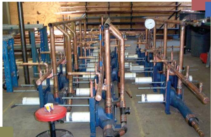
*Using drafting and CAD design, piping assemblies are efficiently prefabricated before they are installed at their final location.*
