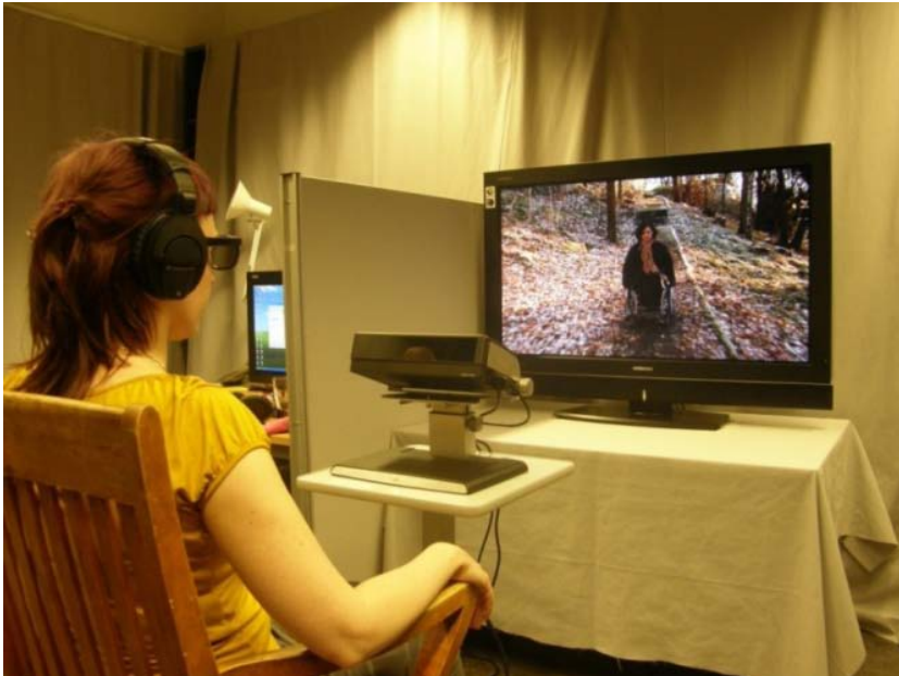
Figure 1. The experimental setting with Hyundai stereoscopic display and Tobii X120 eye movements tracker.
