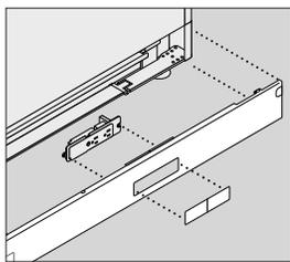
**Panels** are shipped with base covers that have receptacle knockouts.
