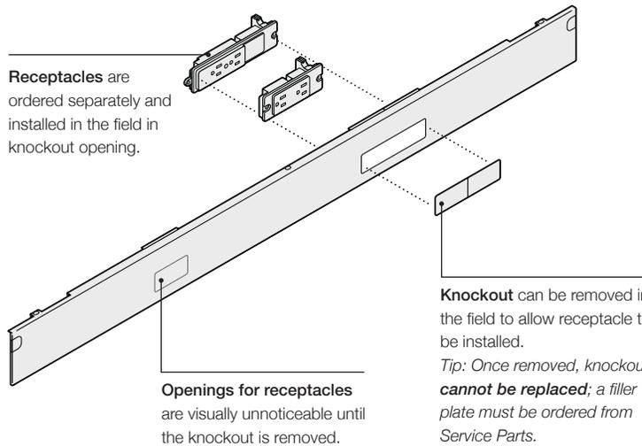
**Receptacles** are ordered separately and installed in the field in knockout opening.
