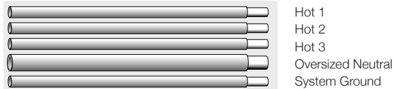
3 Circuit Shared Neutral, 5 Wires
