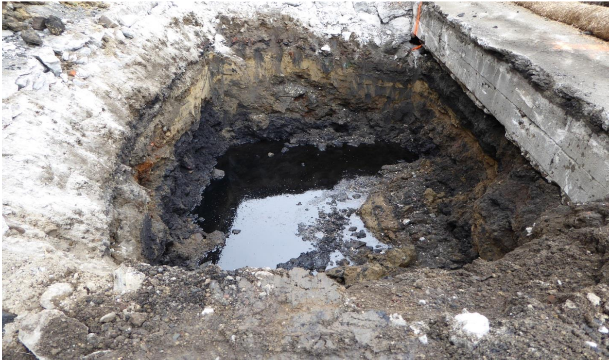
Photo 5 – View of TP-1 looking north, depth approximately five to six feet below top of concrete surface. Photo taken at approximately 1 PM, as the tide is coming in.
