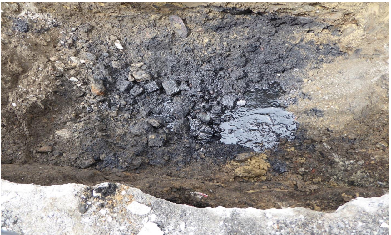
Photo 4: View of bottom of test pit – depth approximately four feet below top of concrete surface. Note presence of oily soils, brick debris and water infiltration.
