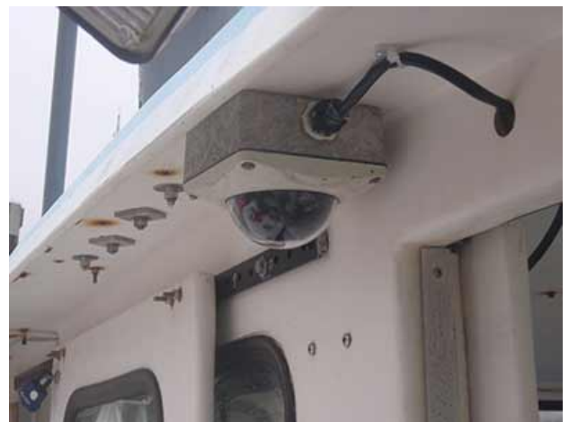
Electronic monitoring camera mounted on a commercial fishing vessel. – Photo courtesy of NMFS
