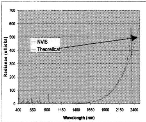
**Figure 2a** Calibration of NVIS spectrometer data using tungsten lamp and integrating sphere.
