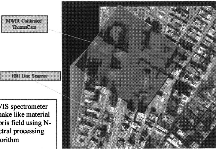
**Figure 5.** High resolution line scanner and calibrated ThermoCam mosaic
