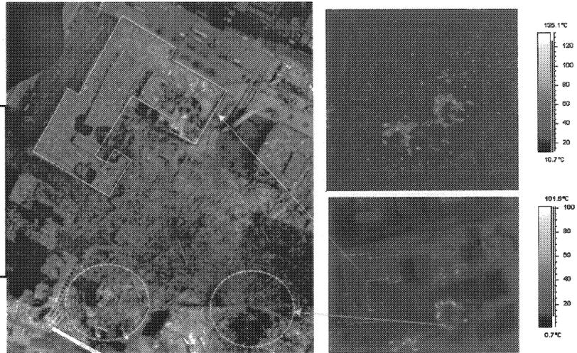
**Figure 4.** High resolution line scanner imagery on left, Thermo Cam 3-5um calibrated temperature data on right. OEM GIS infrastructure overlaid
