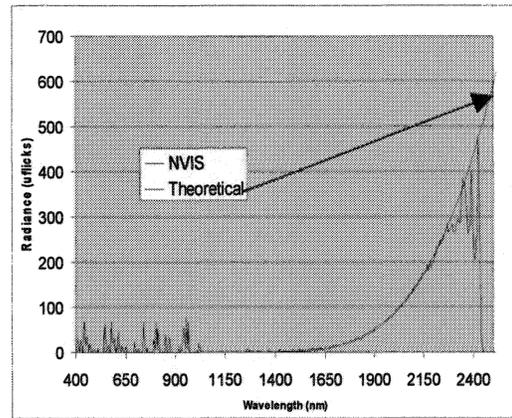
**Figure 2b** Calibration of NVIS spectrometer data using tungsten lamp and integrating sphere for wavelengths below 1.0µm and a large black body source for wavelengths above 1.0µm
