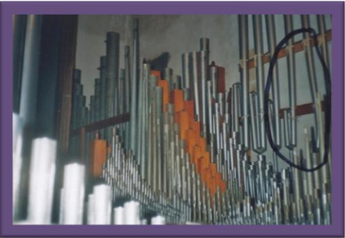
Metal fatigue of slender zinc bass pipes.
