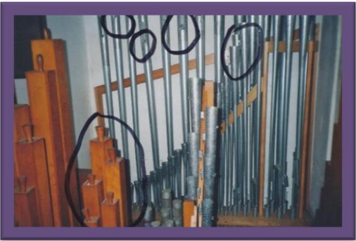
Failing tuning scrolls and wood pipes – tuning stoppers.
