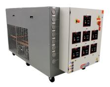
7-zone custom water temperature control system designed for leading pet food manufacturer. Common NEMA 4 rated electrical enclosure with common supply and return for customer supplied chilled water.
