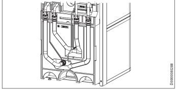
► Release the sensor lead from the guide groove in the insulation segment.
