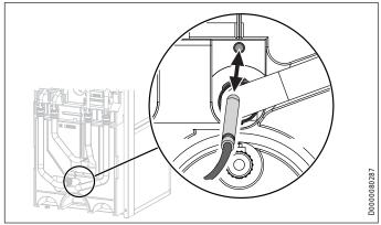
▶ Pull the "heating sensor" out of the buffer tank.
