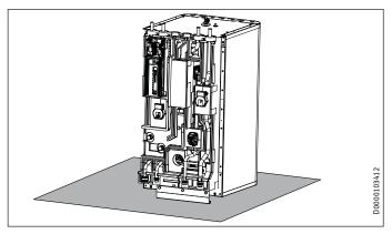
Place the upper section of the appliance on a base to prevent damage.
