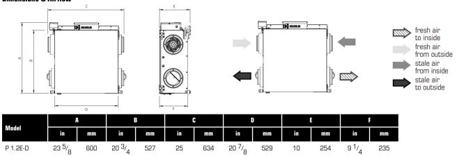
Clearance of 8.5 in. (216mm) in front of the appliance is recommended for removal of core. All appliances feature three foot plug-in power cord with 3-prong plug.
