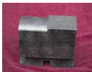
Combination Fullering to flat die
