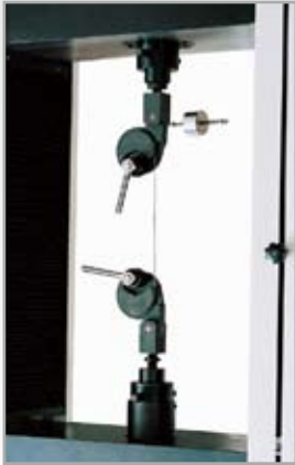
Soft Steel Wire Tension
