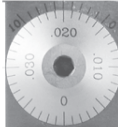
Vernier Scale with Reference Marks. (See page 145)
