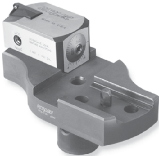
Finish Assembly with attached Finish Head shown here.
