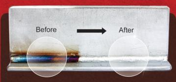
Welding of stainless steel produces a discoloration on the surface that must be removed to improve its apperance and to restore the corrosion resistance of the stainless steel.
