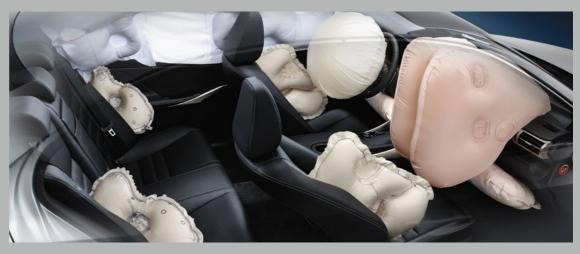
**TEN STANDARD AIRBAGS** The comprehensive safety of the IS ensures every part of the cabin is covered, with side curtain and knee airbags for the driver and front seat passenger and rear outboard-seat side airbags.
