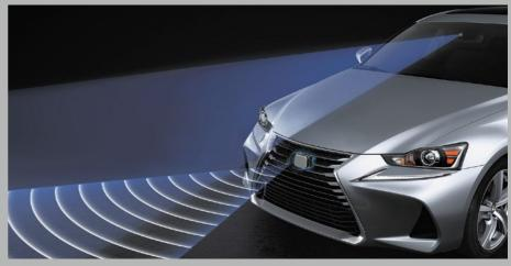
**DYNAMIC RADAR CRUISE CONTROL**<sup>®</sup> & **PRE-COLLISION SYSTEM**<sup>®</sup> An advanced cruise control system maintains a constant speed and adjusts the vehicle's speed depending on the surrounding traffic. The Pre-collision System utilizes a millimeter-wave radar sensor to provide collision avoidance or collision mitigation support in speed ranges where frontal collisions are likely to occur.
