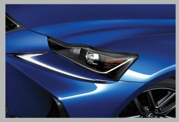
**AUTOMATIC HIGH BEAM**<sup>13</sup> Light your way as necessary, thanks to an in-vehicle camera sensor that assesses the brightness of streetlights, the lights of oncoming and preceding vehicles, and automatically turns the high beams on or off as conditions dictate.
