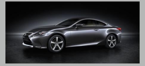
$\begin{tabular}{ll} YIELD TO NOTHING The RC is the truest of coupes: a short wheelbase, a stiff and rigid frame, and a direct-injected 3.5-litre V6, unleashing a maximum 307 horsepower at 6400 rpm with a peak torque of 277lb-ft at 4800 rpm. It also keeps things steady with double wishbone suspension in the front and multi-link suspension in the rear. \\ \end{tabular}$
