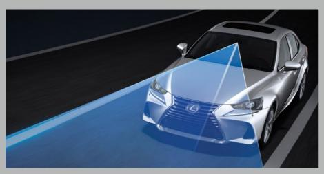
**LANE DEPARTURE ALERT**<sup>4</sup> While your eyes are set on the road ahead, a camera works as a sensor to recognize lane markings around you, alerting when the vehicle deviates from its lane.
