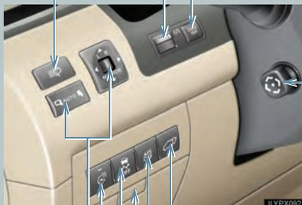
Tilt and telescopic steering control switch P. 100
