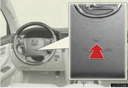
To sound the horn, press on or close to the
