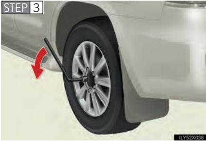
Slightly loosen the wheel nuts (one turn).
