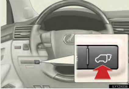
The power back door can be opened/closed using the power back door switch or wireless remote control. (→P. 46)
