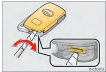
Remove the depleted battery.
