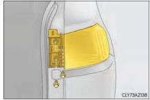
Push and pull the light unit toward the rear of the vehicle as shown in the illustration to remove it.
