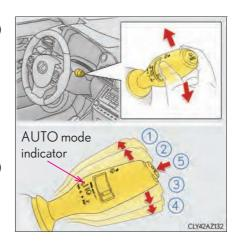
With AUTO mode selected, the wipers will operate automatically when the sensor detects falling rain. The system automatically adjusts wiper timing in accordance with rain volume and vehicle speed.
