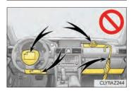
Do not attach anything to areas such as a door, windshield glass, side door glass, front or rear pillar, roof side rail and assist grip.
