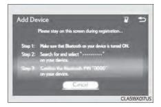
A PIN code are not required for SSP (Secure Simple Pairing) compatible Bluetooth  $^{\circledR}$  devices. Depending on the device, you may need to select Yes to register, or No to cancel on the device.
