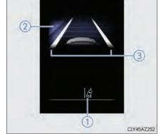
Indicates that steering wheel assistance of the steering control function is operating.
