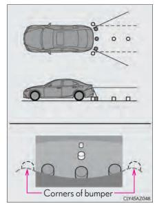
The camera uses a special lens. The distance of the image that appears on the screen differs from the actual distance.
