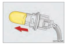
4 Install a new light bulb then install the bulb base to the light unit by inserting it and turning the bulb base clockwise.
