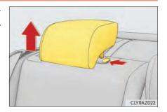
**2** Flip up and fold the cover, and fix it with the hook-and-loop fastener.
