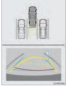
4 Once the vehicle width guide lines and the parking space lines are parallel, straighten the steering wheel and back up slowly until the vehicle has completely entered the parking space.
