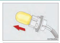
6 Install a new light bulb then install the bulb base to the light unit by inserting it and turning the bulb base clockwise.
