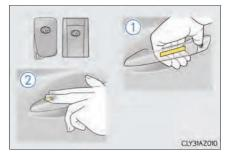
2 Touch the lock sensor (indentation on the upper part of the front door handle) to lock all the doors.
