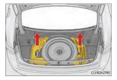
3 Loosen the center fastener that secures the spare tire.
