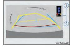
A simplified image is displayed on the upper part of the screen when an obstacle is detected.
