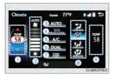
If the "A/C" indicator is turned off, the system will blow ambient temperature air or heated air.
