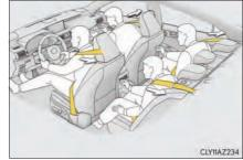
The pretensioners do not activate in the event of a minor frontal impact, a minor side impact or a rear impact.
