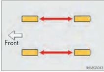
Vehicles with front and rear tires of differing sizes Tires cannot be rotated.
