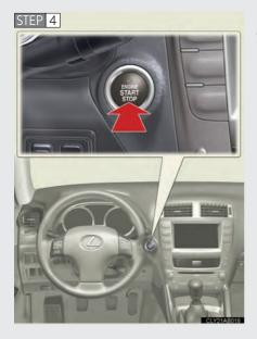
Press the "ENGINE START STOP" switch.
