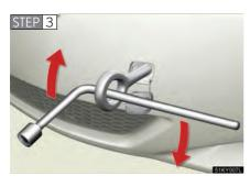
Tighten down the towing eyelet securely using a wheel nut wrench.
