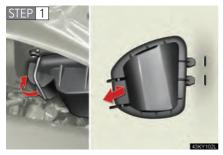
Release the lock and remove the cover.
