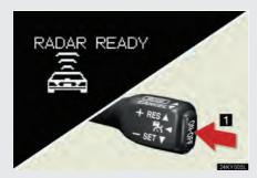
Selecting vehicle-to-vehicle distance control mode
