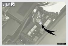
Remove the fuse with the pullout tool.
