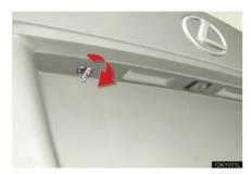
Turn the mechanical key clockwise to open.
