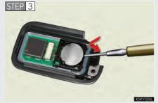
Remove the depleted battery.
