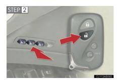
Press and hold the desired button ("1", "2" or "3") while pressing on the wireless remote control until the signal beeps.
