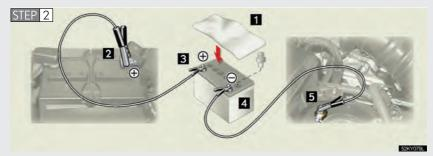
Connecting the jumper cables.
