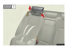
Secure the child restraint using a seat belt or a lower anchors, and lock the head restraint in place at the lowest position.
