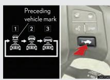
Each push of the switch changes the vehicle-to-vehicle distance
