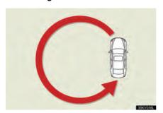
If "CAL" appears on the display, drive the vehicle at 5 mph (8 km/h) or less in a circle until a direction is displayed.
