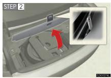
Secure the panel using the hook provided.
