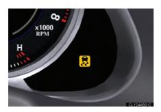
If the vehicle is in danger of slipping, rolling backwards when starting on an incline, or if the rear wheels (2WD) or 4 wheels (AWD) spin, the slip indicator light flashes to indicate that the VSC/TRAC/hill-start assist control systems have been engaged.
