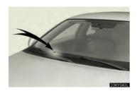
The sensor may not function properly if an object is placed on the sensor, or anything that blocks the sensor is affixed to the windshield.
