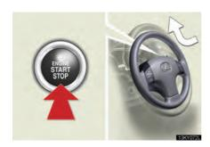
When the "ENGINE START STOP" switch is turned OFF, the steering wheel returns to its stowed position by moving up and away to enable easier driver entry and exit.
