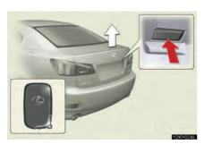
Press the button to unlock the trunk.
