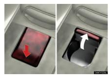
To open, press down and release the front of the cup holder lid.
