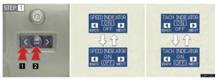
Push < or > to select the speed or tacho indicator set mode. (11) Turn the speed or tacho indicator to "OFF" and then "ON" by pushing the "ON/OFF" button. (21)
