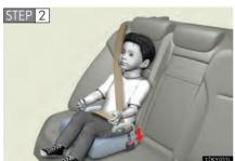
Sit the child in the booster seat. Fit the seat belt to the booster seat according to the manufacturer's instructions and insert the plate into the buckle. Make sure that the belt is not twisted.
