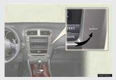
The indicator light flashes after the "ENGINE START STOP" switch has been turned OFF to indicate that the system is operating.
