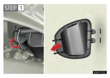
Release the lock and remove the cover.
