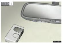
Point the remote control for the device 1 to 3 in. (25 to 75 mm) from the HomeLink<sup>®</sup> control buttons.
