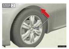
Slightly loosen the wheel nuts (one turn).
