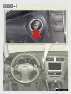
Press the "ENGINE START STOP" switch.
