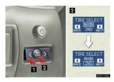
Tire pressure warning valve and transmitter ID code settings display
