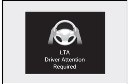
When the lane centering function is operating and the system determines that the vehicle may depart from its lane due to a sharp curve, etc., a warning display urging the driver to operate the steering wheel, will be displayed.
