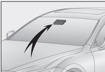
If the system judges that the vehicle is being driven over the speed limit, performing prohibited actions, etc. in relation to the recognized road signs, it alerts the driver using a warning display and warning buzzer\*.
