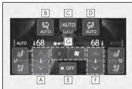
**A** Adjust the left side rear seat temperature setting
