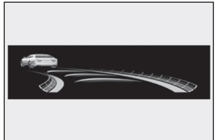
The curve display on the head-up display changes according to the direction and curvature of the curve.
