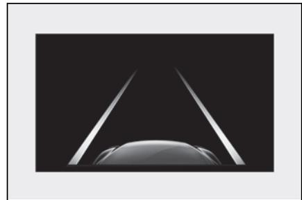
Indicates that the system is recognizing white (yellow) lines. When the vehicle departs from its lane, the white line displayed on the side the vehicle departs from flashes orange.
