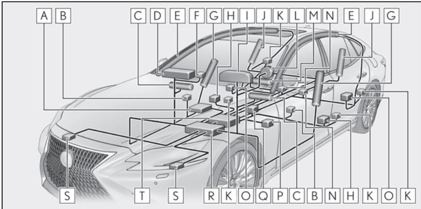
**A** Front passenger occupant classification system (ECU and sensors)
