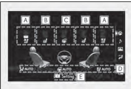
**A** Adjust the seat ventilator fan speed level
