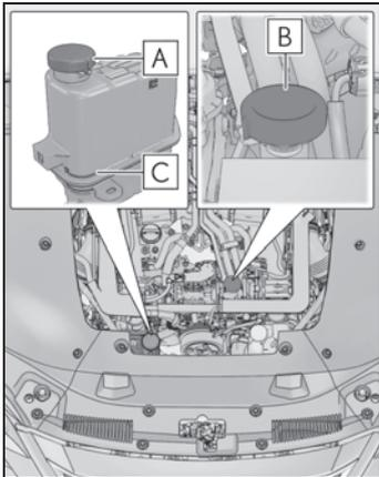
4 Add coolant through the inlet of the cap **A** up to the "F" line **C**, and then replace the cap **A**.
