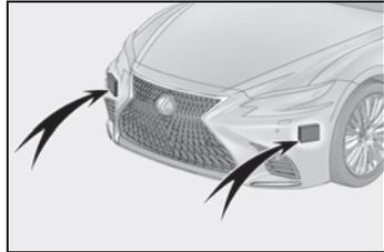
If a radar sensor or its surrounding area on the front bumper is dirty or covered with snow, the system may not operate and a warning message (→P.430) will be displayed.
