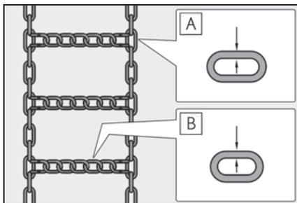
**A** Side chain (0.12 in. [3 mm] in diameter)
