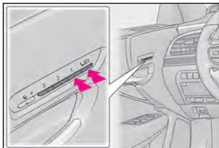
To record the position of the front passenger’s seat, adjust the front passenger’s seat to the desired position and perform step 4 using the buttons on the front passenger’s side.
