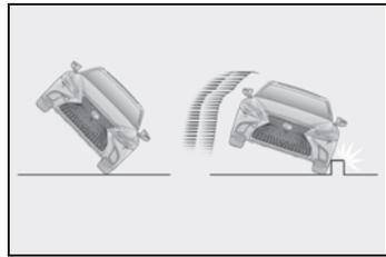
■ **Types of collisions that may not deploy the SRS airbags (SRS front airbags/SRS seat cushion airbags)**
