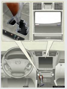
Advanced parking guidance system will activate when the shift lever is in "R" position.
