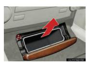
Holding the left edge of the non smokers box, pull upward.
