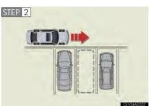
Move your vehicle slowly to a position perpendicular to and as close as possible to the target parking space.
