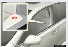
The indicator light flashes after the "POWER" switch has been turned OFF to indicate that the system is operating.
