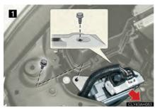
11 Remove the securing bolts and move the ECU.
