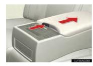
Press the button to release the lock, and slide the lid back.
