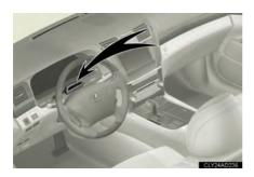
Detects the direction the driver is facing. The system determines whether the driver is facing forward.
