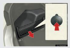
Remove the 12-volt battery cover after removing the clip.
