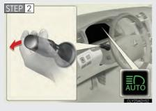
The Automatic High Beam indicator will come on when the headlights are turned on automatically to indicate that the system is active.
