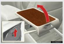
When returning the table, pull it up while pulling the lock release lever.
