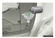
If any washer does not work or the warning message appears on the multi-information display, the washer tank may be empty. Add washer fluid.
