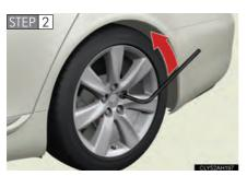
Slightly loosen the wheel nuts (one turn).
