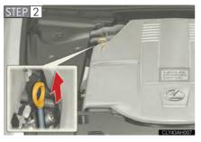
Hold a rag under the end and pull the dipstick out.
