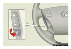
Pull to operate the voice command system. (→"Navigation System Owner's Manual")
