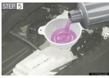
Add power control unit coolant if necessary.
