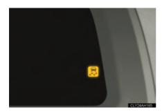
If the vehicle is in danger of slipping, rolling backward when starting on an incline, or any of the drive wheels spin, the indicator flashes to indicate that the VSC/TRAC/hill-start assist control systems have been engaged.
