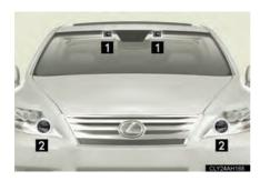
Detect pedestrians and other three-dimensional objects on or near the road ahead together with the radar sensor while the vehicle is moving. When the headlights are on, near-infrared rays are projected to ensure proper detection performance in the night time.
