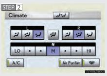
Touch to turn on the windshield wiper de-icer. The windshield wiper de-icer will automatically turn off after approximately 15 minutes. Touching the switch again also turns the de-icer off.
