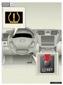
Push and hold the tire pressure warning reset switch until the tire pressure warning light blinks slowly 3 times and a message appears on the multi-information display.
