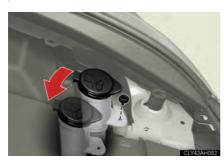
Remove the securing bolt and move the washer fluid filler opening.
