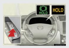
Turns the brake hold system on
