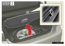
Secure the panel using the hook provided.
