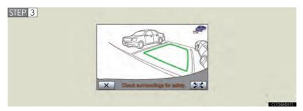
Position yourself as you would when backing up normally, and rest your hands on the steering wheel without applying any pressure. Check your surroundings and behind the vehicle for safety, and slowly back up, using the brake pedal to control the vehicle's speed.
