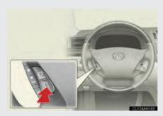
Pressing the pre-support switch while assist mode is on, the "POWER" switch is in ON mode and the vehicle is traveling below 9 mph (15 km/h) with the shift position in any position other than "P" or "R", will cause the screen to change in the following order:
