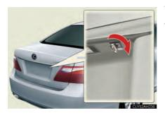
Turn the mechanical key clockwise to open.
