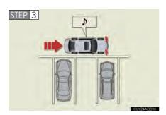
A chime will sound once when the center of the target parking space is visible right beside you. After this chime has sounded, turn the steering wheel about half a turn or more while driving forward.
