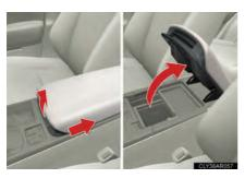
Slide the armrest while pulling up the lever, and lift the armrest.
