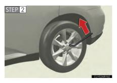
Slightly loosen the wheel nuts (one turn).
