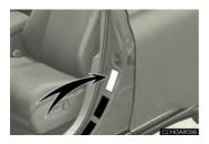
For the GAWR, see the Certification Label. For the maximum load of the tire, see the load limit at maximum cold tire inflation pressure mentioned on the sidewall of the tire.  $(\rightarrow P. 633)$
