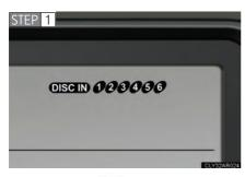
To select the CD to be ejected, press " $\wedge$ " or " $\vee$ " on VTYPE DSC $\wedge$  or
