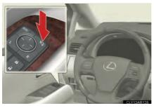
Press the switch to fold the mirrors.
