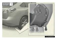
Remove the bolts using a Phillipshead screwdriver, and remove the clip.
