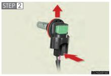
Unplug the connector while pressing the lock release.
