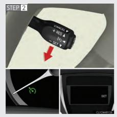
Accelerate or decelerate the vehicle to the desired speed, and push the lever down to set the speed.
