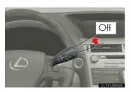
Set the wiper switch to off. If the wiper switch is in "AUTO", the wipers may operate unexpectedly in the following situations, and may result in hands being caught or other serious injuries and cause damage to the wiper blades.
