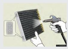
If the filter is dirty, clean by blowing compressed air through the filter from the underside.
