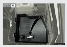
Remove the fuse with the pullout tool.
