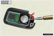
Remove the depleted battery.
