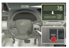
Pressing and holding the head-up display main switch for more than 2 seconds changes the display to audio display on/off mode. Press the head-up display main switch to turn the audio display on/off.
