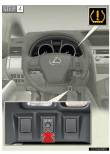
Press and hold the tire pressure warning reset switch until the tire pressure warning light blinks slowly 3 times.
