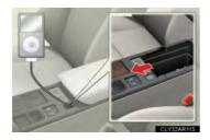
When the cover is slide open, portable audio device cables can be pulled through the opening.
