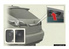
Press the button to unlock the door.
