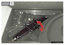
Remove the jack after removing the hook.
