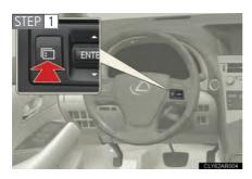
Press and hold the menu switch of the multi-information switches to display customization mode.
