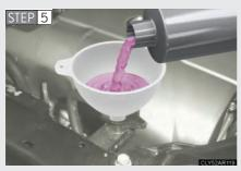
Add engine coolant if necessary.
