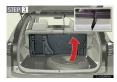
Pull the folded deck board upright, and use the hook to secure the deck board as shown in the illustration.
