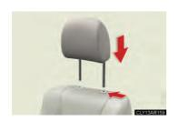
Align the head restraint with the installation holes and push it down to the lock position.
