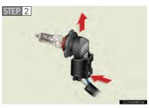
Unplug the connector while depressing the lock release.
