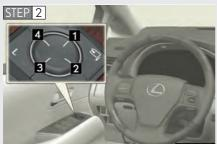
To adjust the mirror, press the switch.
