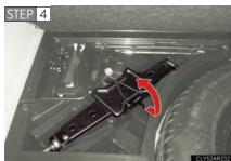
Remove the jack after removing the hook.
