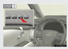
Press button "1", "2" or "3" until the signal beeps to recall the desired position.
