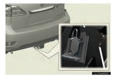
With towing package: Use the wire harness stored in the rear end under body.
