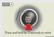
Stop the engine by pressing and holding the "ENGINE START STOP" switch for 3 consecutive seconds or more.
