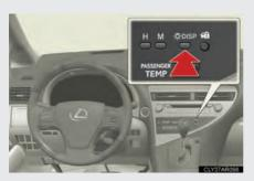
Press and release the "DISP" switch until the brightness of the display is adjusted to the desired level.
