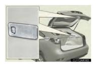
The luggage compartment lights turn on when the back door is opened with the luggage compartment light switch on.
