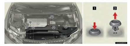
■ Installing the clips
