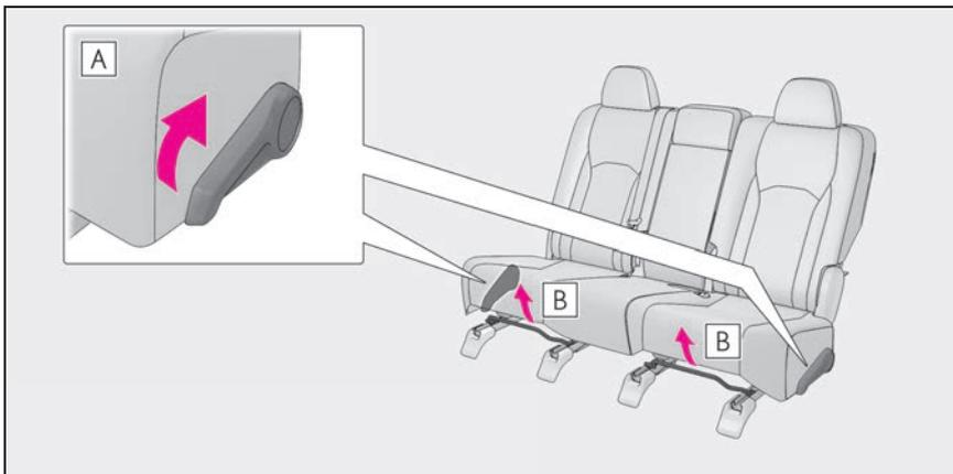
**A** Seatback angle adjustment lever**B** Seat position adjustment lever
