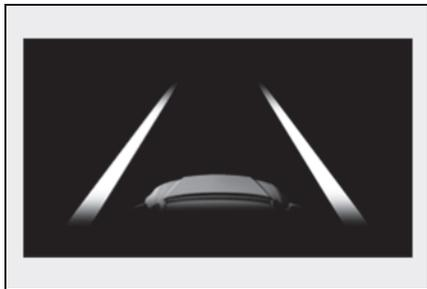
Indicates that the system is recognizing white (yellow) lines or a course<sup>\*</sup>. When the vehicle departs from its lane, the white line displayed on the side the vehicle departs from flashes orange.
