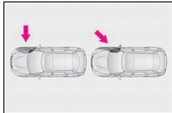
The SRS side airbags do not generally inflate if the vehicle is involved in a frontal or rear collision, if it rolls over, or if it is involved in a low-speed side or low-speed frontal collision.
