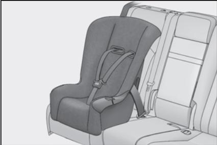
An illustration showing a child seat installed on a car seat. The seat belt is buckled across the child seat. The child seat is positioned on the passenger side of the car seat.                                                                                                                                                                                            | P.50 |
