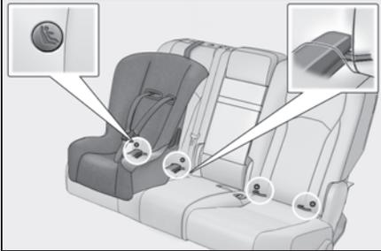
An illustration showing a child seat installed on a car seat using LATCH anchors. The child seat is positioned on the passenger side of the car seat. The LATCH anchors are attached to the child seat's base. Callouts show the LATCH anchors and the LATCH anchors on the car seat. The LATCH anchors on the car seat are located on the seat's backrest and seat cushion. | P.54 |
