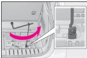
If the spare tire still cannot be lowered, the wire cable may be severed. Have the vehicle inspected by your Lexus dealer.
