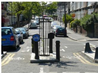
Areas where motor traffic cannot cut through side streets, while walking and cycling are encouraged. By using bollards, planters, or trees, a residential area can be filtered, so that all parts can still be reached by motor vehicle (for deliveries, or to start or end journeys) but direct routes across quiet zones are only possible by non-motorised modes.
