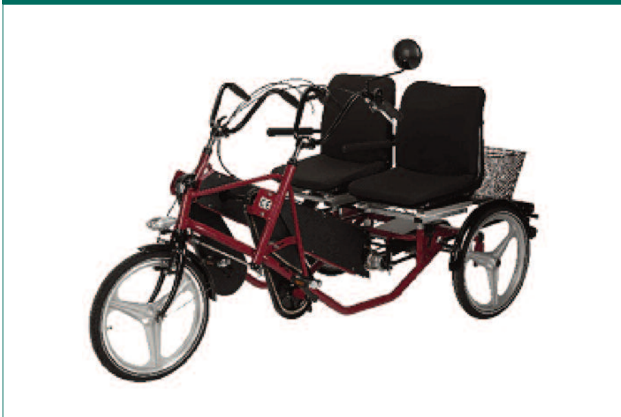
Figure 8.10: Side by side semi-recumbent trike
