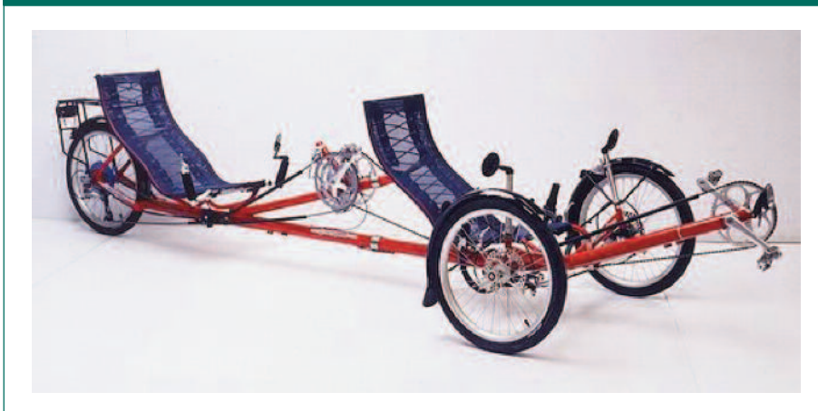
Figure 8.9: Tandem trike with both riders recumbent
