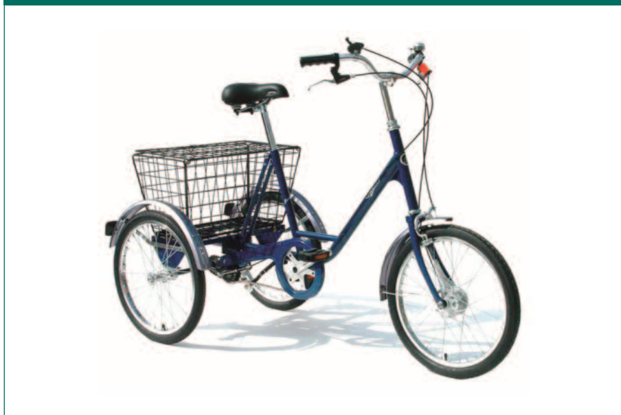
Figure 8.3: Upright trike with two rear wheels and one front wheel Copyright: Pashley Cycles
