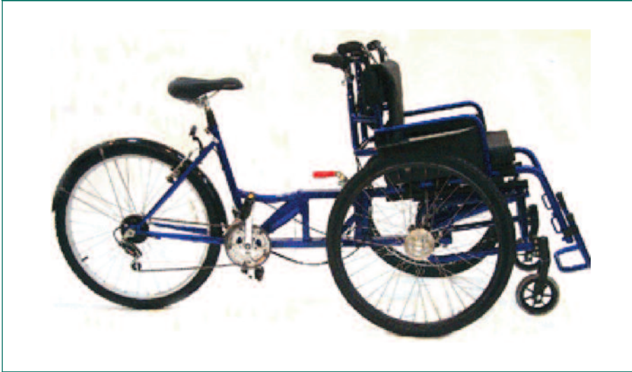
Figure 8.11: Wheelchair tandem (with detachable wheelchair) Copyright: Da Vinci
