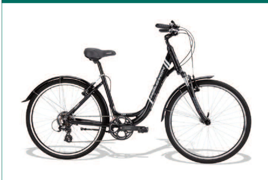
Figure 8.1: Low step-through frame bike
