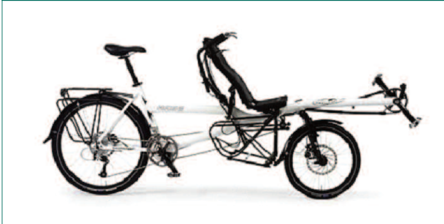
Figure 8.2: Tandem with recumbent front seated rider
