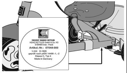
On outdoor play equipment, the label will be located on one of the main beams and/or support bars.
