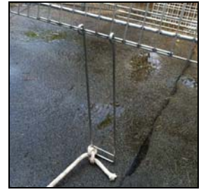
4. Prop bar in raised position
