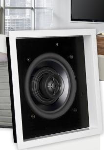
Size 5.65 dia w x 6 d (in) 144 dia x 152 d (mm) Freq Response 100Hz-20kHz±3dB Impedance 4 ohms Sensitivity 86dB 2.83V / 1m Power req. 25-100 watts Woofer (1) 3" (76 mm) Aluminum Tweeter (1)0.75" (19 mm) Aluminum Finishes White Paintable Grille PCB FXC320S-PB (1) 3" (76 mm) Aluminum Cone Driver (1) 0.75" (19 mm) Aluminum Dome Tweeter
