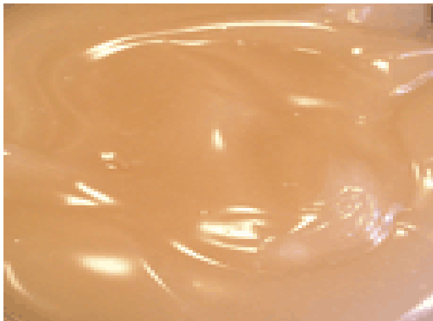
Bulk emulsion, ammonium nitrate solution in oil with stabilizers
