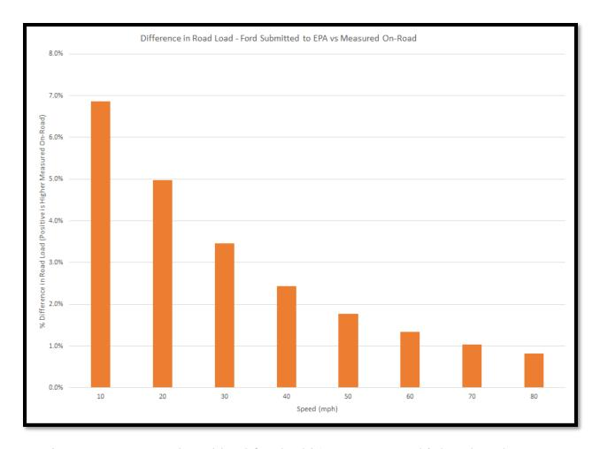
60. Because actual road load for the 2019 Ranger was higher than that used by Ford during certification (and provided to EPA), fuel economy from the vehicle would have been overestimated during certification fuel economy testing, and using the road load derived from actual on road experiments will produce worse fuel economy estimates than those listed on the Monroney label.
