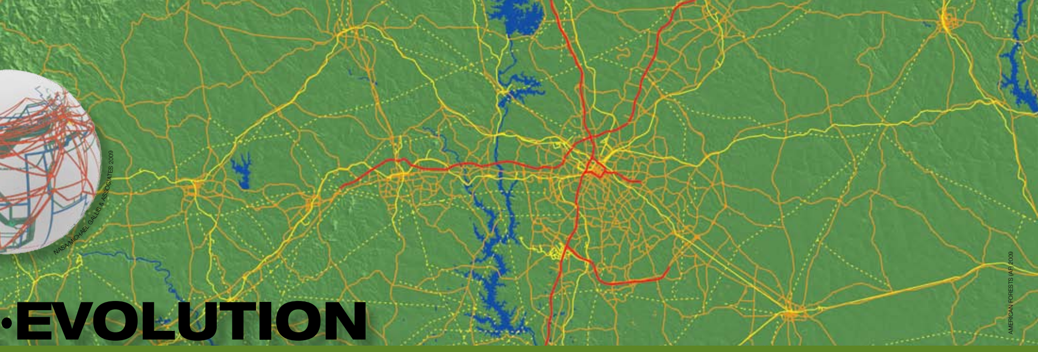
ABOVE: Detail of the network diagram showing the Charlotte, NC region, from the Piedmont Crescent Study. It illustrates the pattern and density of road traffic in red and orange lines. Railroads in yellow lines; power lines in dotted yellow lines. ABOVE LEFT: The sphere at left represents the Natural System; the one at right, the Human Network. Human Network demand for resources from the Natural System creates impacts that lead to de-evolution. Increasingly, these changes in Natural System patterns affect the Human Network.
