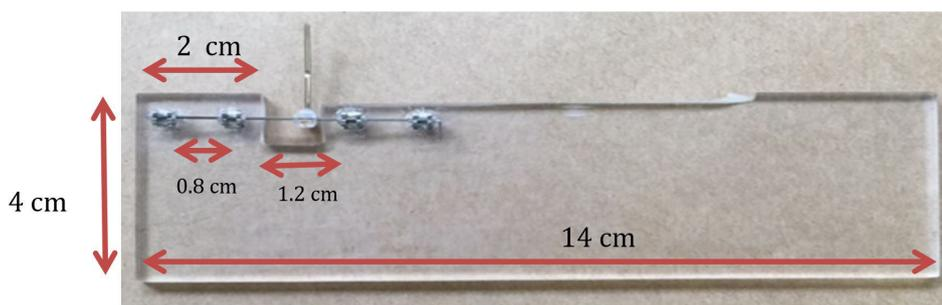
Figure 1. Acrylic plate with brackets positioned for the traction test.
