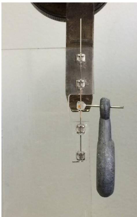
Figure 2. Friction test with conventional metal bracket.
