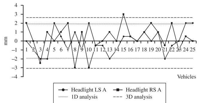
**Figure 10.** Correlation between calculations in one and in three dimensions with measurements in the assembly line for the frontend example.
