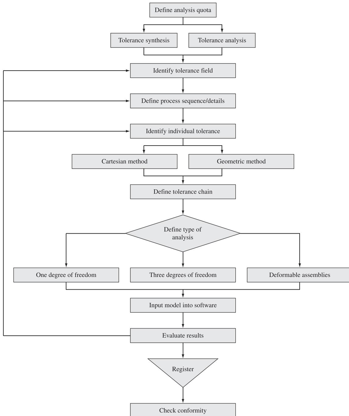
**Figure 3.** Tolerance analysis process.
