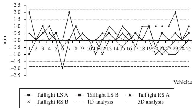
**Figure 9.** Correlation between calculations in one and in three dimensions with measurements in the assembly line for the taillight example.
