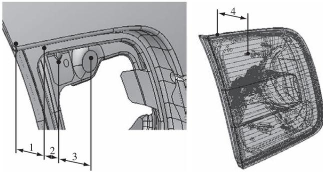
**Figure 7.** Tolerance chain.
