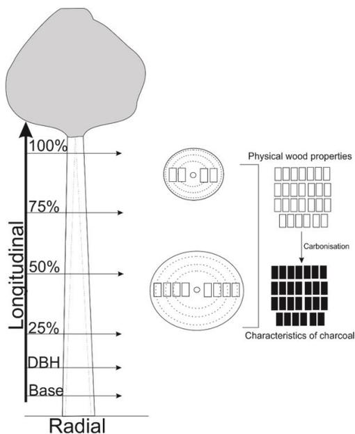
**Figure 1.** Longitudinal positions of wood discs and radial position of the samples.
