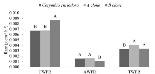
**Figure 1.** Water flow rates in short logs of clones A and B of *E. urophylla* and *C. citriodora*. Where, FWFR is the free water flow rate; AWFR is the adsorbed water flow rate; and TWFR is the total water flow rate. Means followed by the same letter do not differ significantly at 5% probability for the Scott-Knott test.
