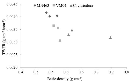
**Figure 3.** Relation between total drying and basic wood density of clones A and B of *E. urophylla* and *C. citriodora*.
