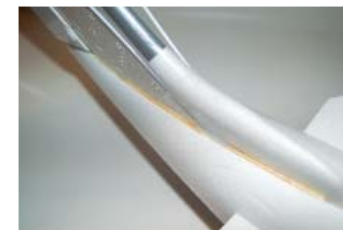
The vertical stabilizer required a few balsa shims to get a snug fit in the fuselage. I applied a fillet of drywall spackle to hide the evidence.
