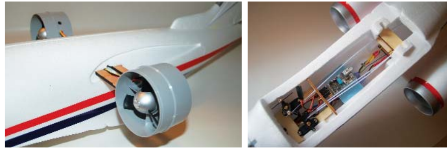
Above left: Hobby Lobby's recommended motors for the Executive Jet fit the EDF units perfectly. The foam nacelles are held in place with tape to facilitate maintenance and repairs. Right: a shelf made of scrap foam makes a handy place to mount the receiver and separate it from the two ESCs. Their rearward position helps establish the CG.
