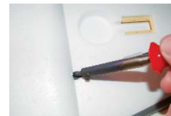
A low-wattage soldering iron is useful for making clean holes through the wing for servo wires and pushrods. Just make sure your workshop is well ventilated.
