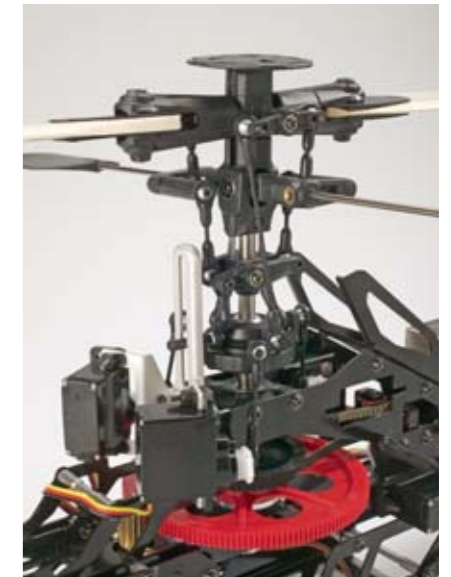
The unique rotor head has an adjustable Bell-Hiller mixing ratio for three different settings. The mildest setting is good for general hovering and flying while the most responsive setting is for radical 3D.
