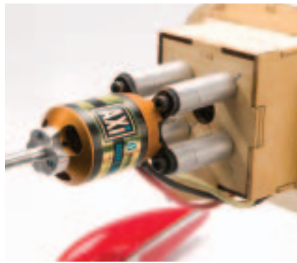
I used aluminum standoffs from Hobby Lobby to mount the Axi Gold motor solidly.
