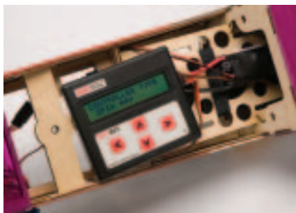
The Jeti "Spin Box" is a powerful tool that's used to program the Spin ESC and retrieve flight data.
