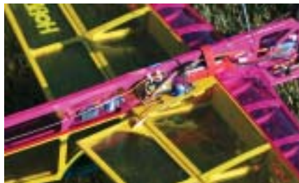
The fuselage has pockets for the servos and battery, a great help for a clean radio installation. A few zip ties hold the wires in check, and keep them out of the control linkages.
