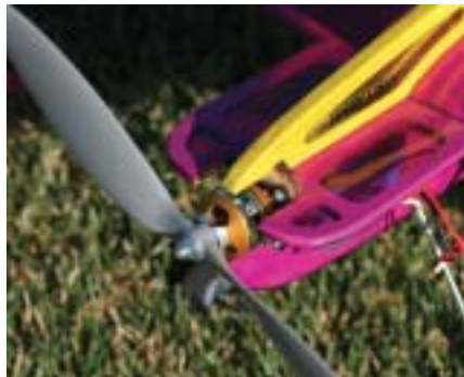
The lightweight laminated motor mount ties into the leading edge of the wing and fuselage sides. The AXI 2208 provides ballistic vertical performance with great acceleration and punch out from hover.
