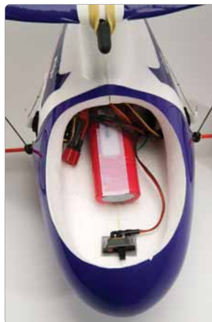
There is plenty of room in the radio bay for all the electronics. Velcro secures not only the battery to the bay but also the cockpit to the battery.
