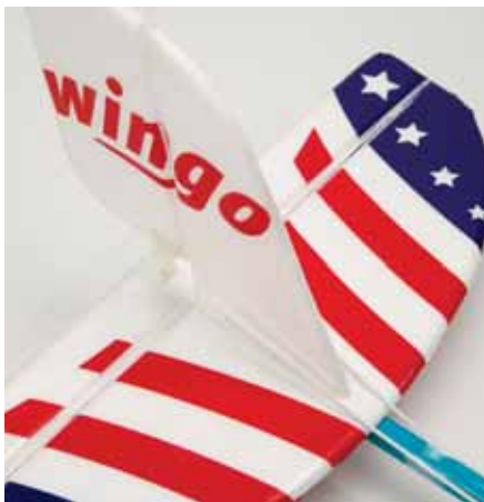
The foam tail feathers are mounted to the sturdy aluminum boom with epoxy.
