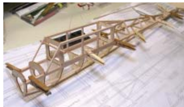
The upper and lower fuselage sections are held together temporarily with a few clothespins.
