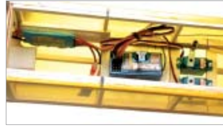
With the wing removed, the servos are visible in the radio compartment near the wing's trailing edge; the receiver is in the center, and the Jeti ESC is near the leading edge. The receiver and ESC are attached with Velcro®.
