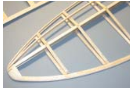
One of the Miss Stik's wingtips. The curved trailing edge is made of three pieces of 1/8-inch-square balsa.
