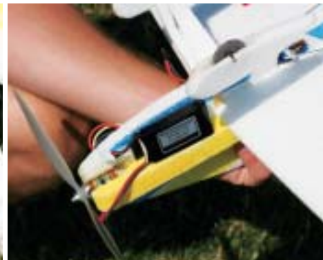
Left: The stock motor mount uses a plywood motor backplate that screws into a ply adapter plate on the firewall. Be careful to follow the directions, as it can be assembled backwards, resulting in left versus the intended right thrust. Right: I prefer to Velcro the battery to the side of the fuselage for maximum cooling and quick battery changes. It would be possible to cut a battery slot into the EPP fuselage if you prefer.
