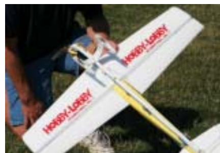
Left: The Super Zoom uses one servo for both ailerons, mounted in the wing center section and connected to the ailerons with short pushrods. You could also use dual aileron servos to add flaperon mixing. Right: Swapping landing gear couldn't be easier—simply slot the prebent gear into the plywood brace and go fly. For those who fly from longer grass, consider removing the gear. Best of all is the floats take only seconds to install when you get to the lake. That kind of versatility is hard to beat.
