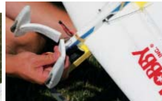
Left: The Super Zoom uses one servo for both ailerons, mounted in the wing center section and connected to the ailerons with short pushrods. You could also use dual aileron servos to add flaperon mixing. Right: Swapping landing gear couldn't be easier—simply slot the prebent gear into the plywood brace and go fly. For those who fly from longer grass, consider removing the gear. Best of all is the floats take only seconds to install when you get to the lake. That kind of versatility is hard to beat.
