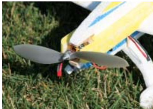
Left: The stock motor mount uses a plywood motor backplate that screws into a ply adapter plate on the firewall. Be careful to follow the directions, as it can be assembled backwards, resulting in left versus the intended right thrust. Right: I prefer to Velcro the battery to the side of the fuselage for maximum cooling and quick battery changes. It would be possible to cut a battery slot into the EPP fuselage if you prefer.
