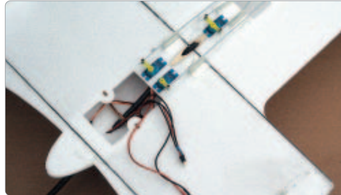
Above left: precisely molded foam parts make the assembly process easy. Above right: it's important that the RC gear be installed and working properly before you glue the lower hull into place.
