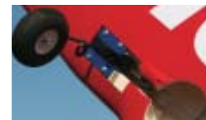
Retracts come with the T-6 kit from Hobby Lobby, and are easy to install and operate.
