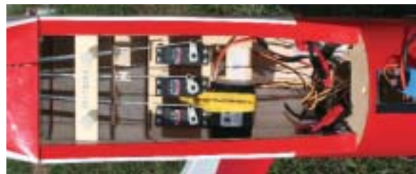
The fuselage has plenty of space for installing the radio, but you will need to tuck the batteries as far forward as possible to establish the proper balance point. I used a split pack installation.
